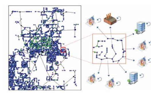
This example of a distribution system used in the Distributed Energy Systems Simulator includes the distribution network itself and models of price-responsive network users connected to each node. The network users can react to expected future price signals by changing their short-term behavior and by adopting DER technologies.
