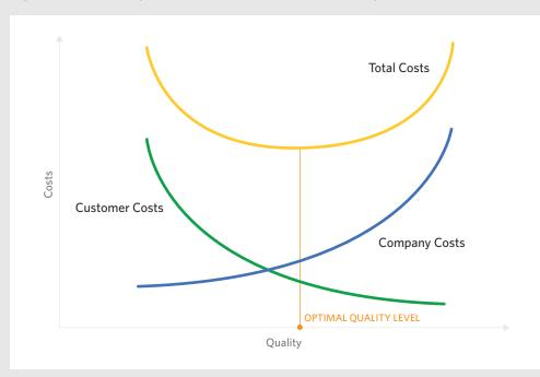
Figure 5.3: Initial Optimal Level of Performance Quality
