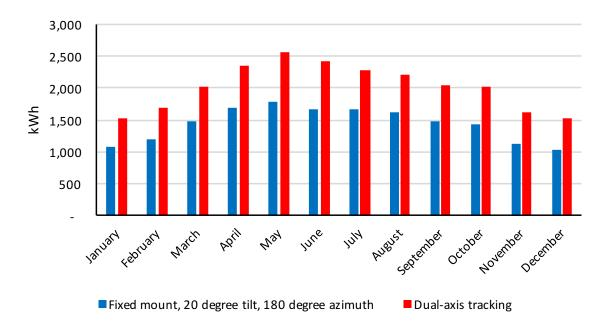
Figure 2.2: AC Energy Produced by 10-Kilowatt c-Si PV Systems in Phoenix, Arizona, Deploying Different Mounting Systems
