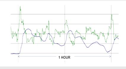
Figure 7.6: Regulation Signals for Two Secondary Reserve Products in the PJM System
