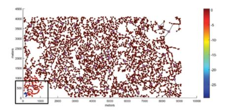
4.13c: Node voltage (per unit) in a zoomed-in section of the network shown in 4.13a
