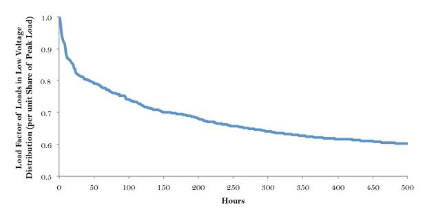
Figure 8.10: Load Duration Curve for Top 500 Hours of Demand in a Low-Voltage Distribution Network (Spanish Example)<sup>18</sup>
