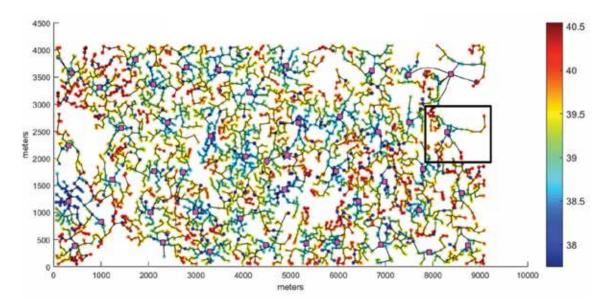
4.11b: Distribution-level active power nodal prices along a small fraction of the network connected at a single MV/LV transformer
