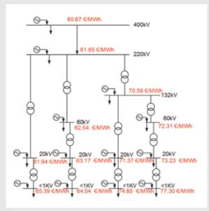
4.9b: Marginal prices for 9 a.m. during a day in April when the Spanish system had a penetration level of solar PV connected at low voltage (under 1 kV) providing 35 percent of total generation capacity
