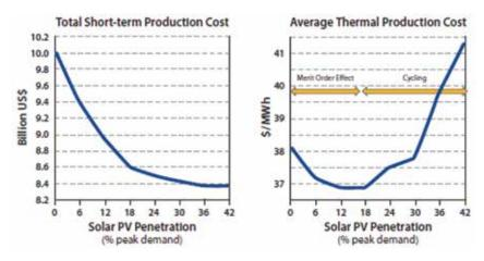
Note: The figure shows total short-term production cost and average short-term production cost for thermal generators only associated with increasing solar penetrations in ERCOT, a thermal-dominated system. (MIT 2015)
