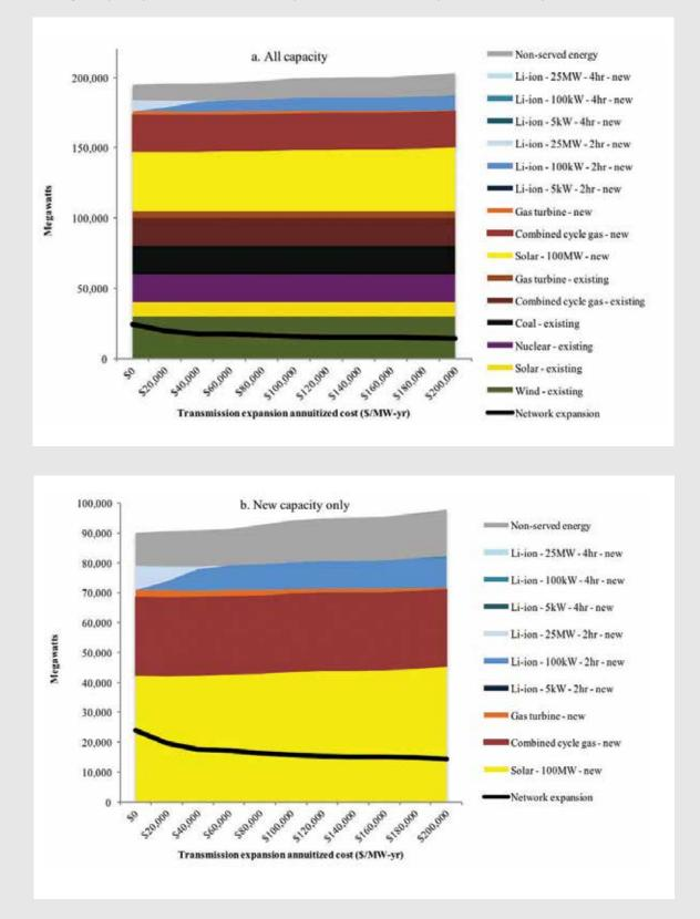
Figure 8.24: Effect of Transmission Expansion Cost on the Optimal Generation and Energy Storage Capacity and Transmission Expansion Decisions (Spain-like Test System)
