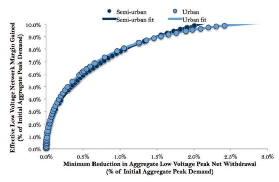
Figure 8.8: Potential for DERs to Substitute for Network Upgrades in Representative European Distribution Networks (Low-Voltage Distribution Example)
