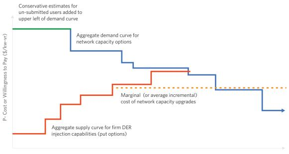
Q- Firm Network Capacity or Firm DER Injection Capability (kW)
