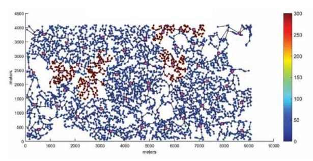
Figure 4.12: Spatial Variation in Distribution-Level Active Power LMPs Caused by Network Congestion in the Network of Figure 4.10
