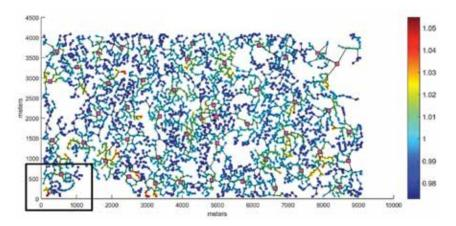
4.13b: Spatial variation of distribution level reactive power LMPs (dollars per megavolt-ampere reactive per hour)
