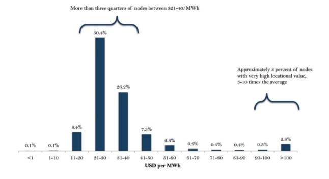
The situation depicted in Figure 4.6 is not an unusual one. **Figure 4.7** shows the distribution of the annual average LMP value at each locational node of the PJM system in 2015. This distribution provides clear evidence of the need for a locational characterization of the energy prices in the PJM system. Similar differences in the marginal price of energy at different locations are observed in other power systems.
