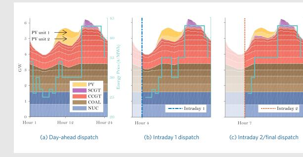
Figure 7.1: Sequential Dispatches as PV Output Is Corrected and Corresponding Intraday Prices
